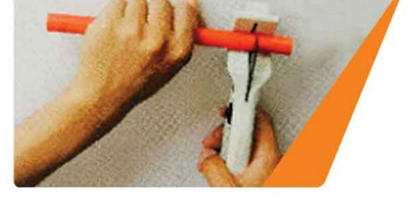
2.Insert the tube into the corresponding reamer, gently rotate the tube on removing the burrs at the front of the tube, and it will shows the corresponding marks line on the surface of the tube (to verity if the tube is well inserted).
