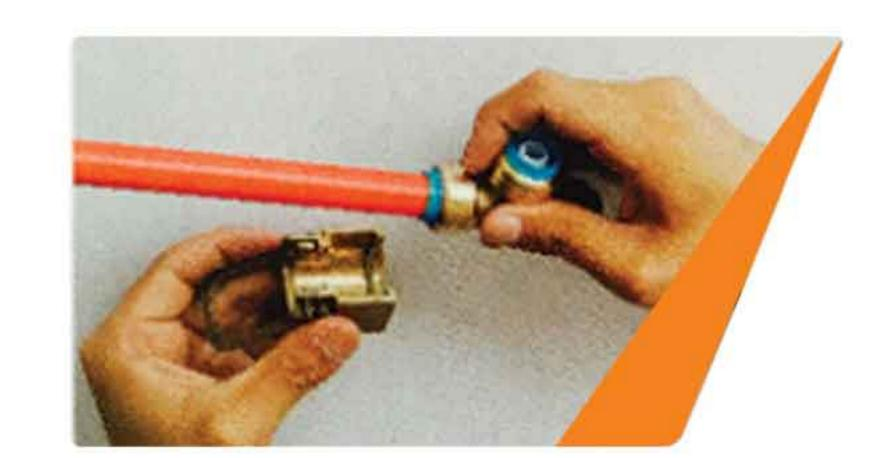
2.Apply firm pressure to the clip, forcing it against the release collar of the fitting. Twist and pull the applicable tube while maintaining pressure on the disassembly clip to release the tubing from the push fitting.
